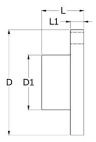
$\begin{array}{lll} D & = 198 \\ D1 & = 120 \\ L & = 80 \\ L1 & = 20 \\ Max \ bore & = 70 \\ Torque \ (N \ m) = 1300 \end{array}$
